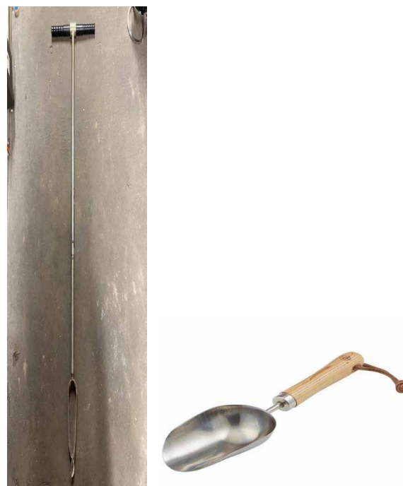
Figure 6.6: Soil auger for soil sampling (0–10 cm) (photo: NIVA) and scoop for soil sampling (Chandra et al., 2024).
