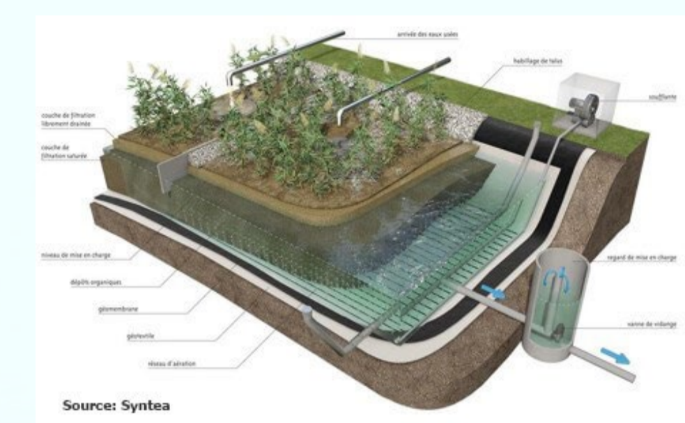
Figure 1. Technical pilot "FR": treatment of raw wastewater and sludge in wetlands. Source: [1].
