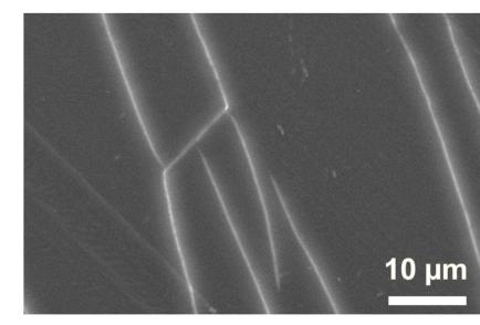
Formation of cracks and surface 10 µm rugosity
